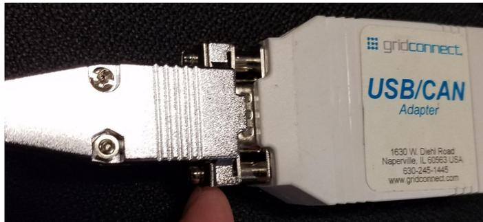
2. Be careful not to apply excessive force to this connection. Check periodically to make sure this connection is secure.
