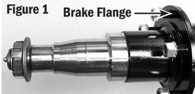
debris or grease, and inspect the bearing surfaces and threads for damage. Carefully inspect the original brake flange for straightness and any weld spatter or imperfections that will affect proper mounting of the brake caliper later (Fig. 1).
